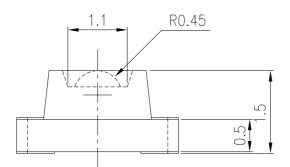
For reflow soldering (propose)
