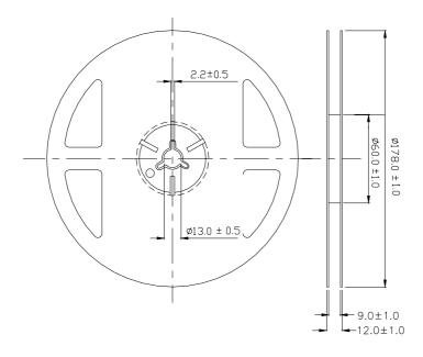
**Note:** The tolerances unless mentioned is  $\pm 0.1$ mm, Unit = mm
