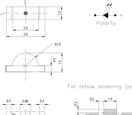
For reflow soldering (propose)
