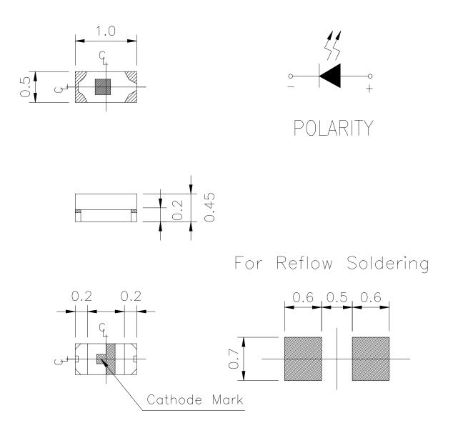
**Note:** The tolerances unless mentioned is  $\pm 0.1$ mm, Unit = mm
