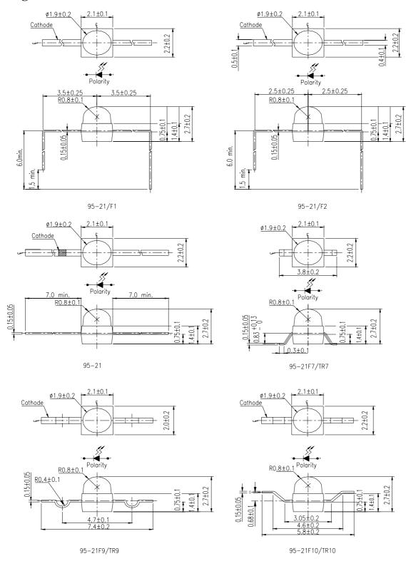
**Note:** The tolerances unless mentioned is  $\pm 0.1$ mm ,Unit = mm
