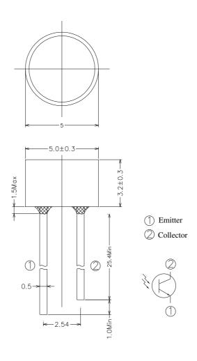
**Notes:** 1.All dimensions are in millimeters 2.Tolerances unless dimensions  $\pm 0.1$ mm
