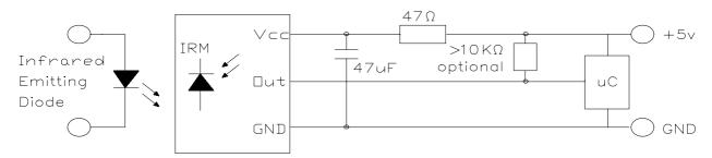
RC Filter should be connected closely between Vcc pin and GND pin.
